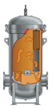
Facet filter housings are specifically designed to remove solid particles such as rust, dirt, pipe scale, sand and metal from fuel. They are commonly located ahead of clay treaters and coalescer separators to protect and prolong cartridge life. A single pass through the filter allows clean product to flow downstream.
