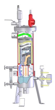
Facet's standard carbon steel VCS Series SuperFlex™ Coalescer Separators are small, economical housings for in-line removal of water and solids from aviation fuels where water content is a problem. Using Facet high quality coalescer and separator cartridges, they provide the best water and solids removal.
