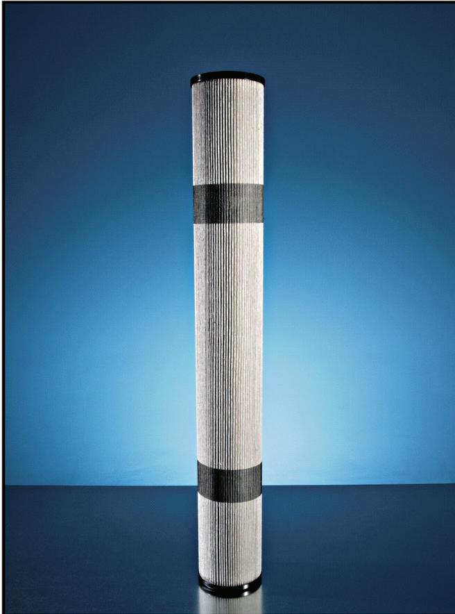
Facet FA Series microfilters offer superior filtration for removing ultra-fine solid contaminants such as rust, scale, granular and other types of solids from aviation fuel systems. They are designed to flow from the outside to inside and qualified at a rate of 4.69 gallons (17.75 liter) per minute per inch of length.
