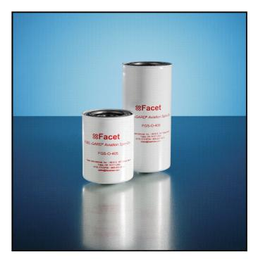
Facet's Fuel-Gard® Aviation Spin-On Filters perform three jobs to give you clean, dry fuel. They absorb free and emulsified water, remove ultra-fine solids even when surfactants and fuel additives are present, and shut down system flow when hit with a localized slug of water. The filters are designed to flow at a rate of 13 gpm (FGS-O-405) and 15 gpm (FGS-O-409).
