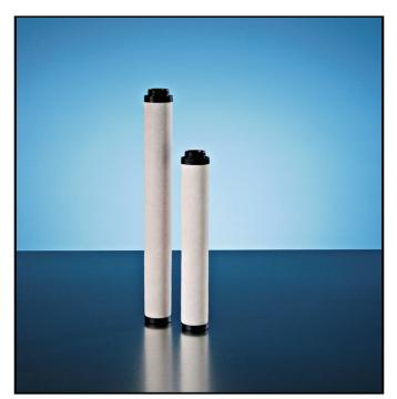
The Facet 2" (51 mm.) nominal outside diameter FG Series Fuel-Gard® monitor cartridges perform three jobs—they absorb free and emulsified water, remove ultra-fine solids and shut down system flow when hit with a localized slug of water, giving you clean, dry fuel. The FG Series Fuel-Gard® monitor cartridges are designed to flow from the outside to inside at a rate of 1 gallon (3.79 liters) per inch of length.
