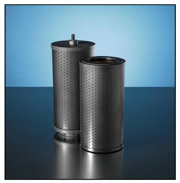
The Facet Flushing Filter elements are designed to be used in place of coalescer elements in a coalescer separator vessel during flushing on new systems or when there's been repairs to the existing equipment. The elements are less expensive than coalescer elements and have more filtration media for better solids holding capacity. Benefits, features and materials of construction are similar to our MP Series filter elements, except designed to flow inside to outside same as coalescer cartridges.
