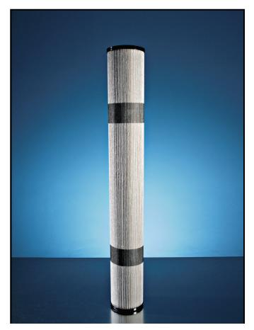
Facet FA Series microfilters offer superior filtration for removing ultra-fine solid contaminants such as rust, scale, granular and other types of solids from aviation fuel systems. They are designed to flow from the outside to inside and qualified at a rate of 4.69 gallons (17.75 liter) per minute per inch of length.
