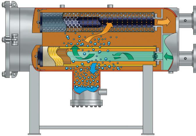
Category M Coalescer Separator housings are for Military JP-8 or JP-5 fuel. Type S qualifications can be used at all filtration points in an aviation fueling system. Type S is meant to be used at filtration points where significant levels of water and dirt in the product can be expected. Facet HCS Series Horizontal Coalescer Separator housings fully comply with EI 1581, Category M, Type S requirements.
