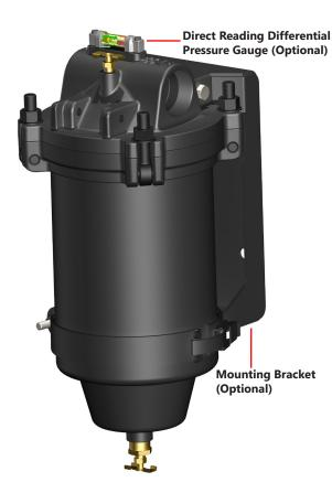
These housings installed with one Fuel-Gard<sup>®</sup> monitor cartridge, will continually check the entire flow of fuel, not just mere samples, for water or solids contamination. By performing three jobs, this small compact monitor assures clean, dry fuel. It absorbs free and emulsified water, removes ultrafine solids, and shuts down system flow when hit with a localized slug of water.
