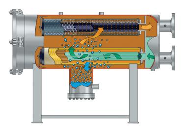
Category M Coalescer Separator housings are for Military JP-8 or JP-5 fuel. Type S qualifications can be used at all filtration points in an aviation fueling system. Type S is meant to be used at filtration points where significant levels of water and dirt in the product can be expected. Facet HCS Series Horizontal Coalescer Separator housings fully comply with El 1581, Category M, Type S requirements.
