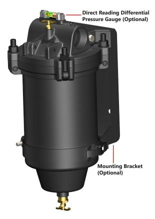
These housings installed with one Fuel-Gard® monitor cartridge, will continually check the entire flow of fuel, not just mere samples, for water or solids contamination. By performing three jobs, this small compact monitor assures clean, dry fuel. It absorbs free and emulsified water, removes ultrafine solids, and shuts down system flow when hit with a localized slug of water.
