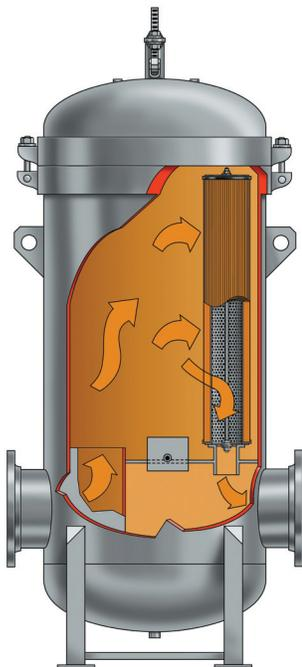
Facet filter housings are specifically designed to remove solid particles such as rust, dirt, pipe scale, sand and metal from fuel. They are commonly located ahead of clay treaters and coalescer separators to protect and prolong cartridge life. A single pass through the filter allows clean product to flow downstream.
