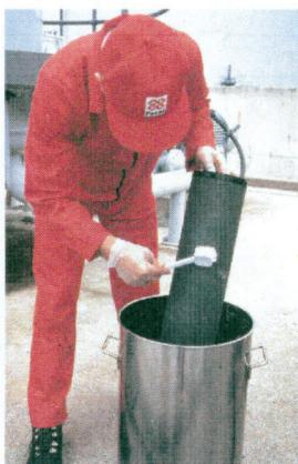
1. **CAREFULLY** remove each element from the filter separator.
